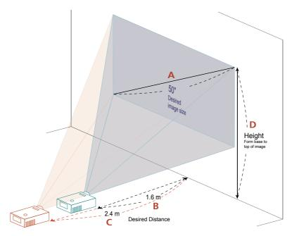
The table below shows how to achieve a desired image size by adjusting either the position or the zoom ring. For example: to obtain an image size of 50" set the projector at a distance 1.6 m and 2.4 m from the screen and adjust the zoom level accordingly.
